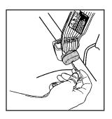
Disconnect the rear center safety belt latch from the mini buckle, if your vehicle has this, by using an object such as a car key.
